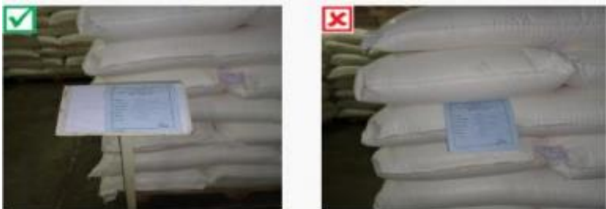
Figure 4: Stand for keeping batch cards for identification and traceability of raw materials
