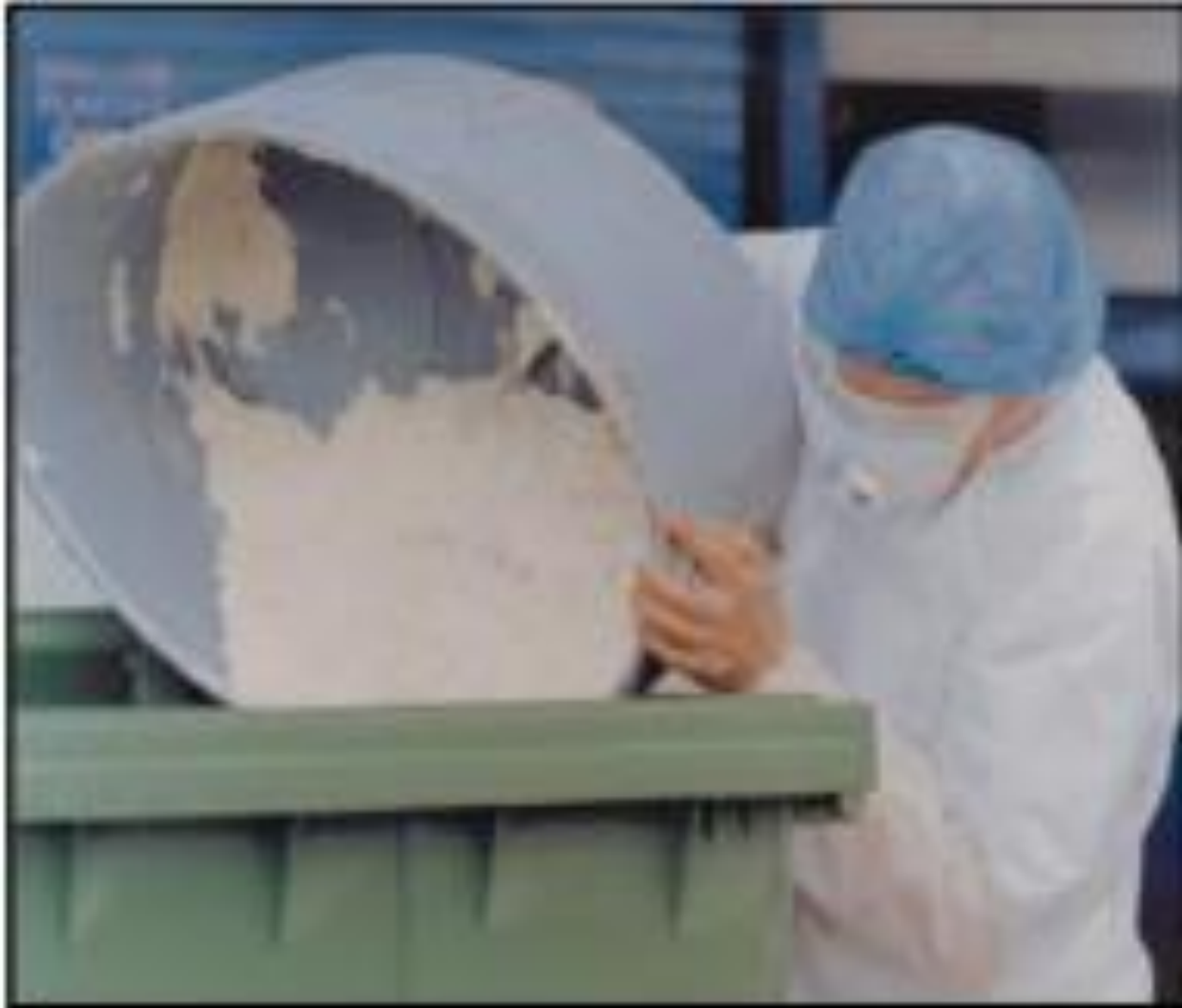
Figure 1: Use of protective clothing and RPE for emptying vacuum cleaner drum
